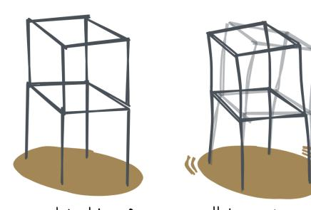
A typical building frame ...will begin to shake made of steel beams... under excitation...
