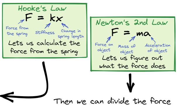
from the springs by the mass to find out the acceleration of the objects. From this we can predict how it'll move.
